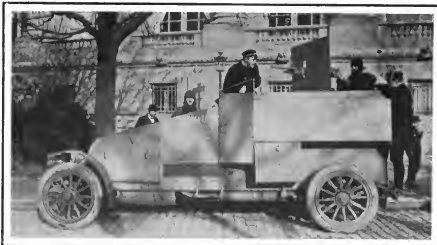
Renault armored automobile manned by French marines. The first series of these cars has just been delivered and taken over by the French naval brigade operating in Belgium. The chassis used is that of the 18-horsepower Renault model, the only change being the alteration of the rear axle to permit mounting dual tires
